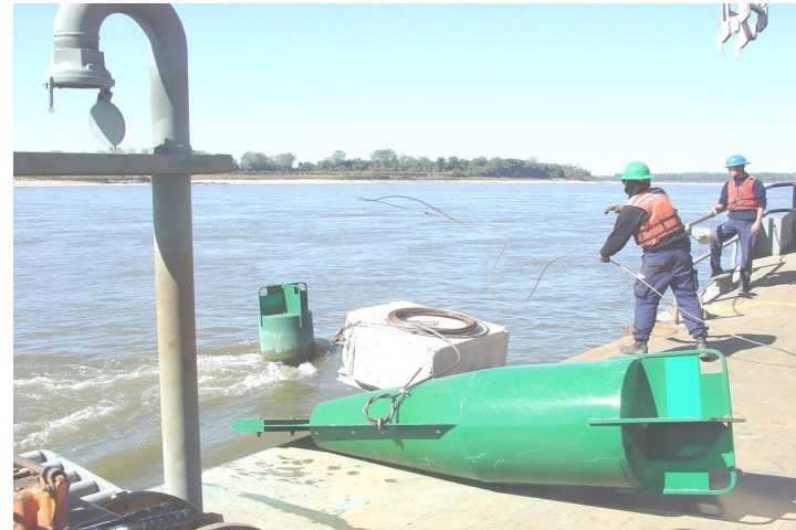
Crew members retrieving a floating ATON and preparing to deploy a new sinker and ATON. Photo provided by USCG.
